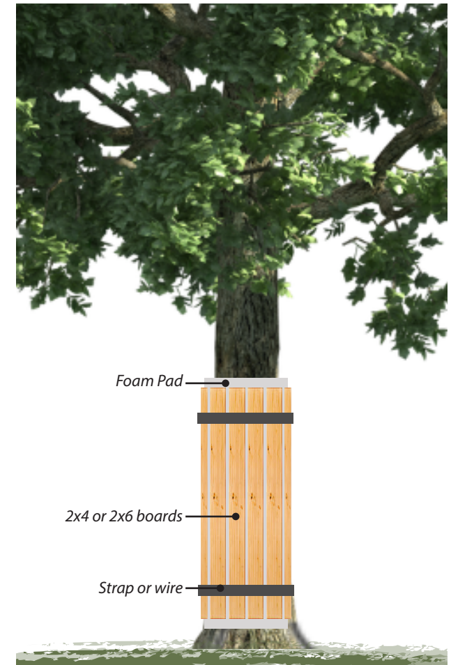
Trunk Protection Structure
