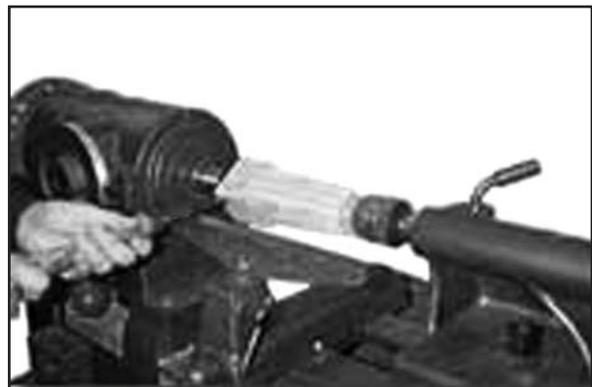
Projected or broken work pieces can be another hazard if not secured between the centers or if the work piece is defective. Furthermore, chuck keys can project if left in the chuck. Flying wood chips from the turning operation also can pose a hazard on wood lathes.
